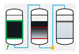
Adding additional vessels in front of the sample point allows the MTZ progression to move through the bed of the first filter and into the second without triggering a media swap. This allows the first bed more operational time, driving it closer to exhaustion.
