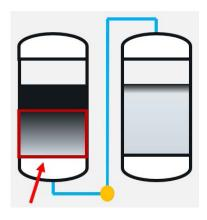
Unused media that will be discarded due to MTZ progression, causing breakthrough between lead/lag vessels before media is exhauseted.
